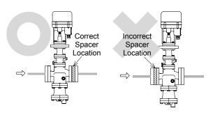
Piping Support Install the MC-COSR, paying attention to avoid excessive load, bending and vibration. Support the inlet and outlet pipes securely.
