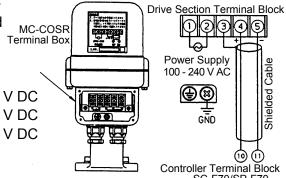
If the value is outside this range, check for disconnected wiring or controller malfunction. If the voltage is correct but the drive section does still not rotate, there may be a malfunction in the drive unit. Refer to "Drive Section Troubleshooting" and take appropriate measures.
