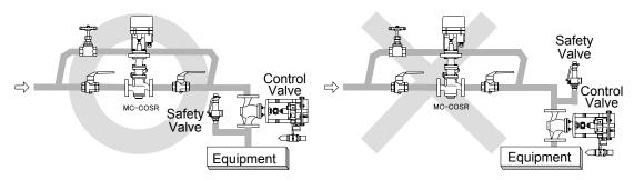
A control valve (i.e. for temperature control) installed between the MC-COSR and the steam equipment (downstream of the MC-COSR) may raise the pressure between the MC-COSR and the control valve when the control valve is closed, depending on their spatial relationship. Therefore, the control valve should be installed close to the steam equipment. Also, a safety valve should be installed downstream of the control valve.
