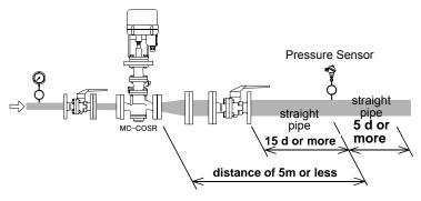
pressure loss and delay of pressure change along this distance will increase, resulting in steam flowrate fluctuations. Steam fluctuations at the pressure sensor may impair the stability of the pressure control. Ensure a straight piping run of at least 15 d upstream and 5 d downstream from the pressure sensor.
