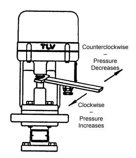
12. If the secondary steam pressure does not change in steps 10. and 11. above, see the **Pressure Reducing Valve Troubleshooting** section.
